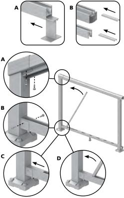
A: Remove the second post to install the last few balusters and spacers.
