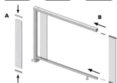
Cut the last spacers flush with the ends of the rails.
