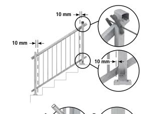
A: Reposition the balustrade panel in between the posts at the required height above the noses of the treads. Place and mark positions of each base rail bracket. Then remove the panel in order to mark hole positions for each bracket on the posts.
