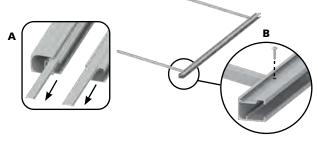
Insert the balusters into each end of the handrail (ensure the screw holes in the rail are facing up). Align the screw hole in each baluster with the screw hole in the handrail, then fasten each baluster to the rail using 12 mm pan head self-drilling screws.
