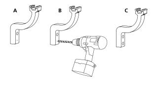
**3.** Measure and mark the position of all brackets on the wall. For timber applications only, use a stud finder to ensure the brackets are located over solid wood.
