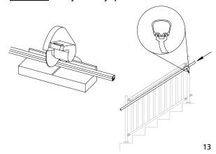
**7.** Once in position, drill a 3.5 mm pilot hole through the bracket and into the handrail. Fasten the bracket to the handrail with a screw (provided).
