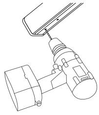
**14.** Secure end caps with screws (provided) at each end of handrail.
