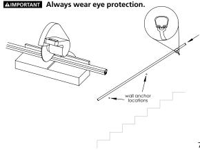
**7.** Once in position, drill a 3.5 mm pilot hole through the bracket and into the handrail. Fasten the bracket to the handrail with a screw (provided).
