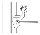
**3.** Drill a 6.5 mm hole through the balustrade post at the marked position.
