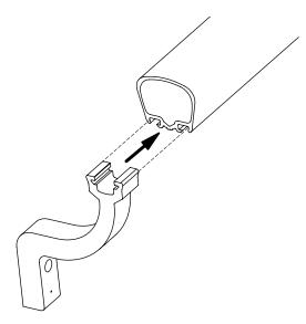
**9.** With the help of another person, adjust the handrail to the desired height and centre the remaining bracket(s) on the balustrade post(s). Mark position of bracket(s) on the balustrade post(s) and drill 6.5 mm hole(s) through the balustrade post(s) at marked position(s). Then follow step 4 to attach the bracket(s) to the balustrade post(s).
