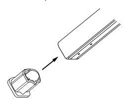
**13.** Drill 3.5 mm pilot holes through handrail and end caps at each end of handrail.
