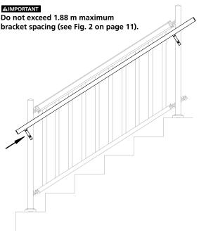
**10.** Follow step 7 to fasten the remaining bracket(s) to the handrail.
