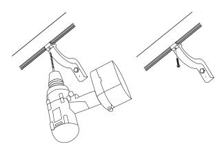
**8.** From the bottom end, slide the required number of brackets into the underside of the handrail.
