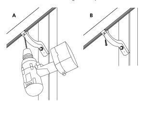
**8.** From the bottom end, slide the required number of brackets into the handrail channel.
