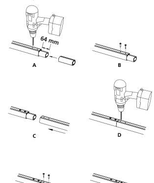
**6.** Measure and cut the handrail to the desired length, then slide the handrail onto the top bracket.
