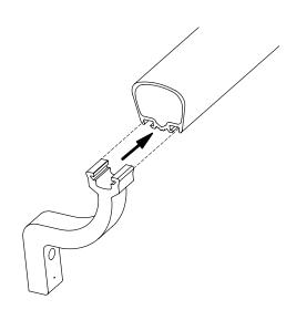
**9.** With the help of another person, adjust the handrail height and slide the bracket(s) into the marked positions. Then follow step 4 to attach the bracket(s) to the wall.
